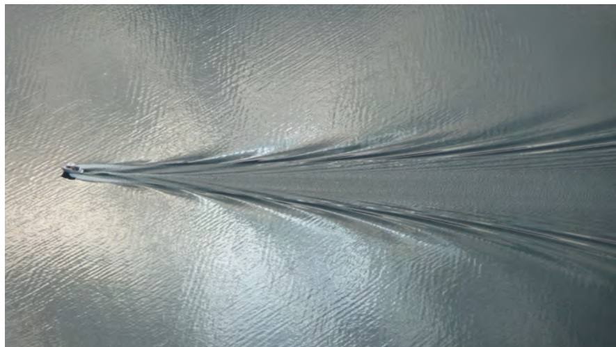
Figure 2. Typical wave pattern of a planning craft.
