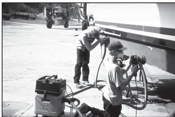
Figure 4-16. Vacuum sanders. Employees at The Lodge of Four Seasons Marina (Missouri) use vacuum or “dustless” sanders to prepare hulls for painting, reducing waste in the environment and cleanup time (USEPA, 1996: Clean Marinas—Clear Value ).
