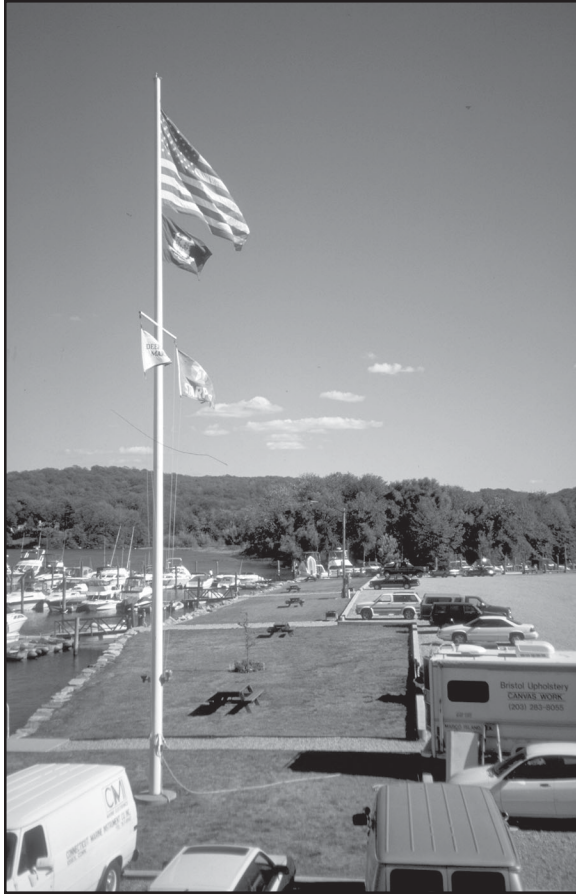
Figure 4-9. Storm water runoff is controlled at Deep River Marina (Connecticut) by 50-foot-wide grass buffers and a parking lot that is covered with crushed rock and has sediment traps in the storm drains. Picnic tables and flowers in the lawn areas make the marina visually attractive and useful to families. Summerfield Boat Works (Florida) added an unpaved parking lot across the street from the main marina property and basin and landscaped its perimeter to blend in with the neighborhood. Harbour Towne Marina (Florida) reduced runoff contamination by planting a grass buffer around the perimeter of the facility. The facility's parking is largely paved and drains to the buffer strip, and the grass adds a cooling and visually pleasing element to the marina property (USEPA, 1996: Clean Marinas—Clear Value ).
